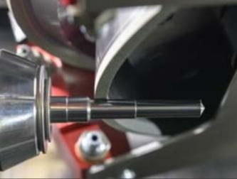
**Swivelling Grinding Unit** Back taper 3°, front taper 10°.
