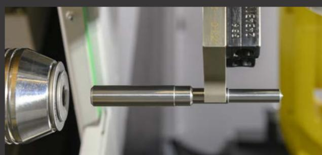
Loading device with up to four pallets. Capacity (example): Shank diameter 10 mm  $[0.4"] \rightarrow 450$  pieces.
