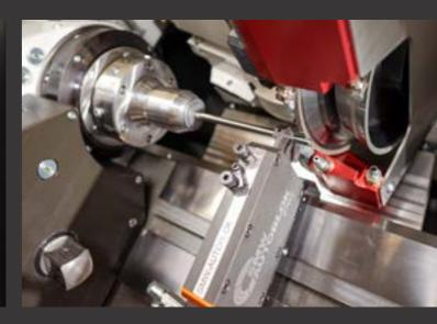
**Dressing** Grinding wheel dressing right inside the machine, simple and precise.
