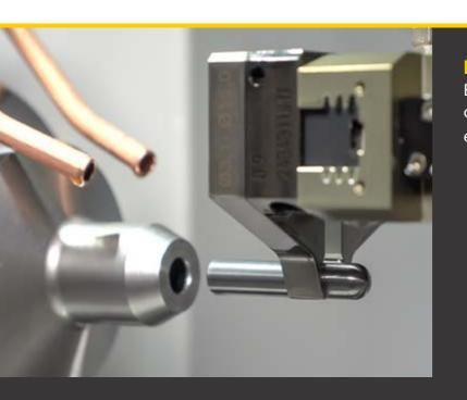
**Pick-up Automation** Easy set-up and reliable changing of the workpieces also in hydraulic expansion chuck.
