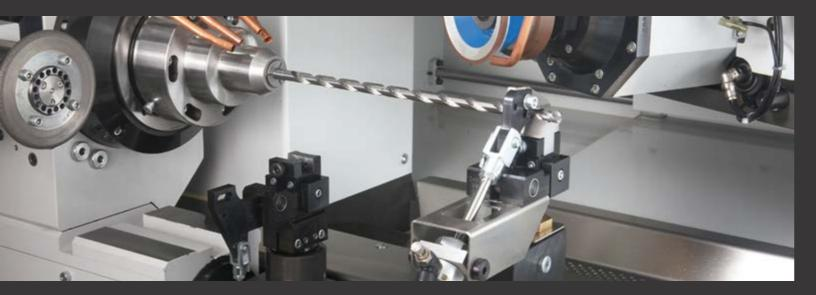
Second Probe Progress integrated measuring of grinding wheels in the machine.
