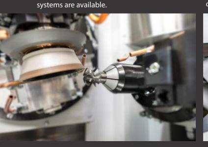
Tail Stock Different versions allow the clamping between centers.
